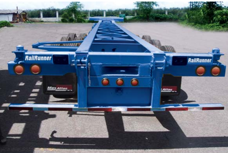
53 FT. SPLINE RAILRUNNER CHASSIS
