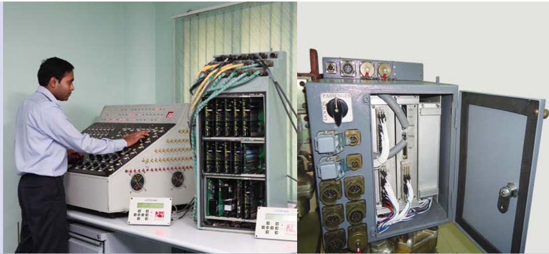
FAULT DIAGNOSTIC AND CONTROL SYSTEM
